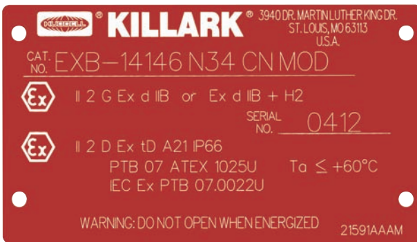
Nameplate for a Certified flameproof enclosure "System" listed to ATEX and IEC Ex Standards for the International Zone System.
